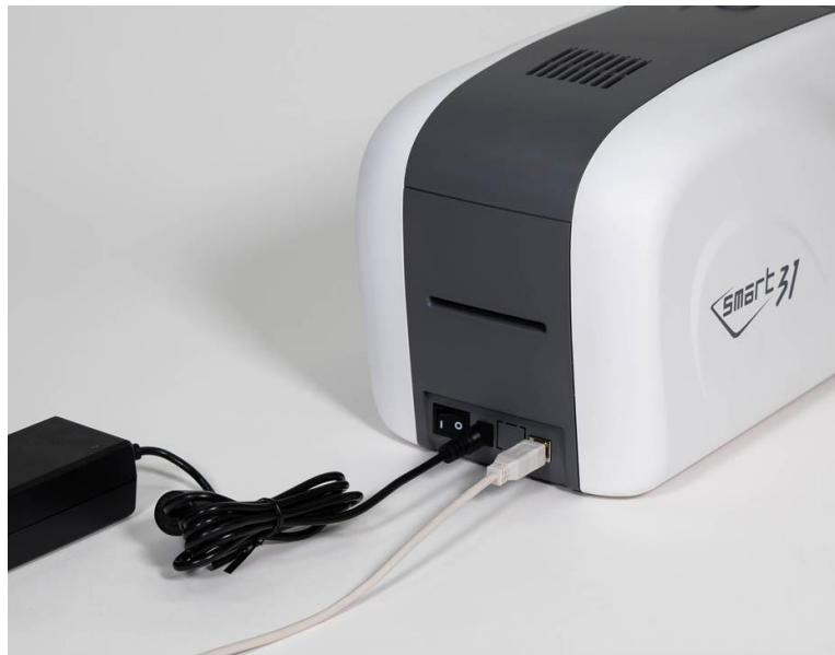
Figure 8 SMART-31S Connection of power and USB cable
