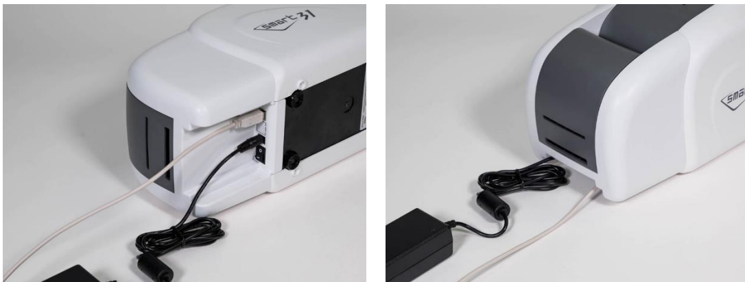
Figure 9 SMART-31D Connection of power and USB cable
